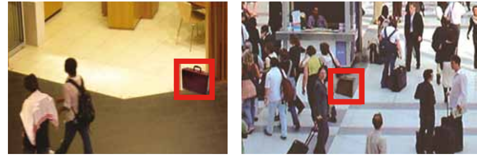
Simple object detection with iQ-100 which is available from many suppliers (Left). Sophisticated object detection in a crowd which is only available from iOmniscient iQ-140, (Right).
